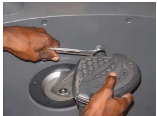
Figure 8 - Loosen right pedal nut
