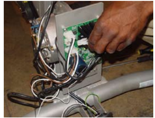
Figure 21 - Disconnect speed sensor cable
