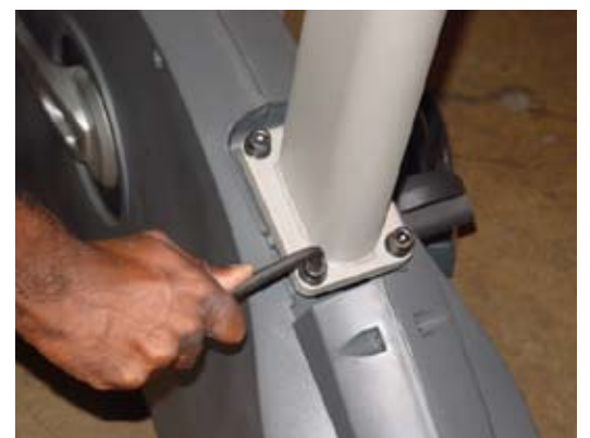
Figure 5a - Unbolt mast from frame (U916)
