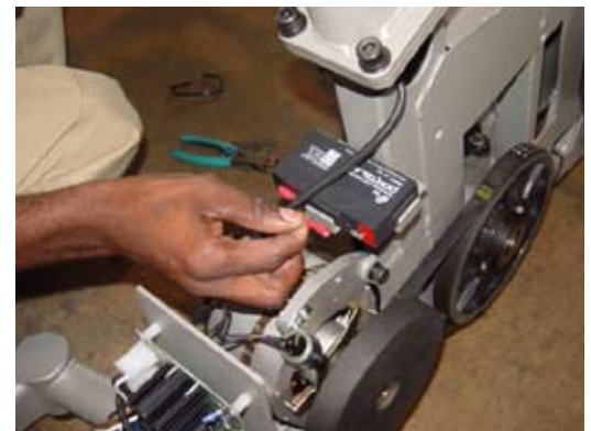
Figure 12 - Disconnect battery cable
