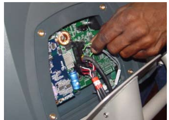
Figure 2 - Cable connections in back of Console (R916 console shown)
