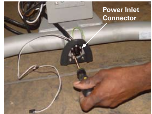
Figure 19a - Remove mounting screws
