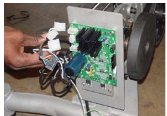
Figure 14a - Disconnect power board cables (U916 shown)
