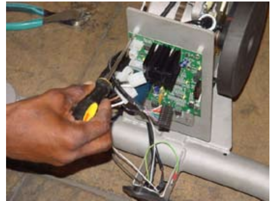
Figure 15 - Power board mounting screws
