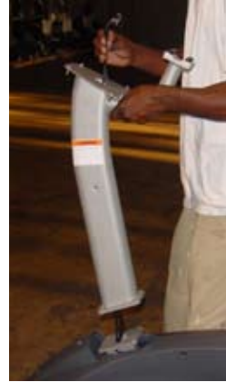
Figure 6a - Lift mast off frame (U916)
