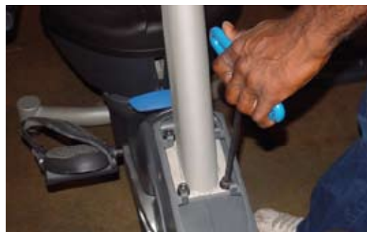
Figure 5b - Unbolt mast from frame (R916)
