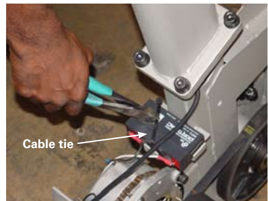
Figure 11 - Cut cable tie
