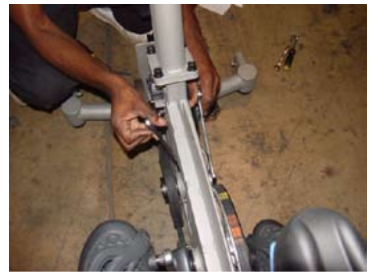
Figure 29a - Loosen belt tensioner
