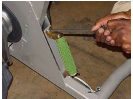
Figure 10a - Unscrew resistor (U916 shown)
