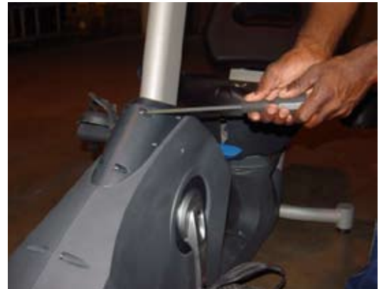
Figure 3b - Remove left mast cover
