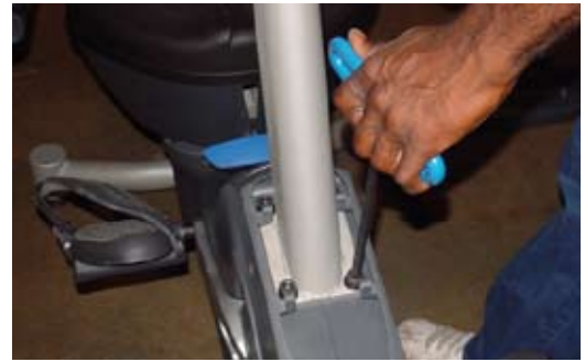
Figure 5b - Unbolt mast from frame (R916)
