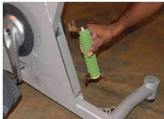
Figure 10b - Remove resistor (U916 shown)
