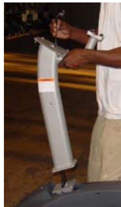
Figure 6a - Lift mast off frame (U916)
